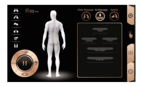
3. **Special function** includes Feet Rollers, Back Heating Vibration function. Press the corresponding button once to start function, press button again to stop the corresponding function.
